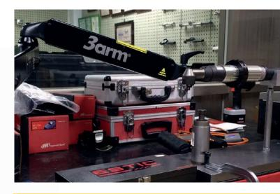
A compact multi-purpose arm for use when brakes are not required
